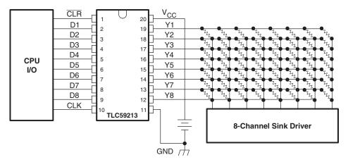
Figure 4. Example of LED Display Connection
